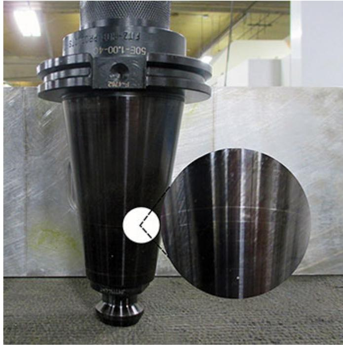
The problem is poorly designed, traditional retention knobs – a less than \$30 part – when tightened create a bulge in the taper that prevents proper seating in the spindle. Once this expansion occurs, the toolholder will not pull fully into the spindle and so cannot make contact with upwards of 70% of its surface.
