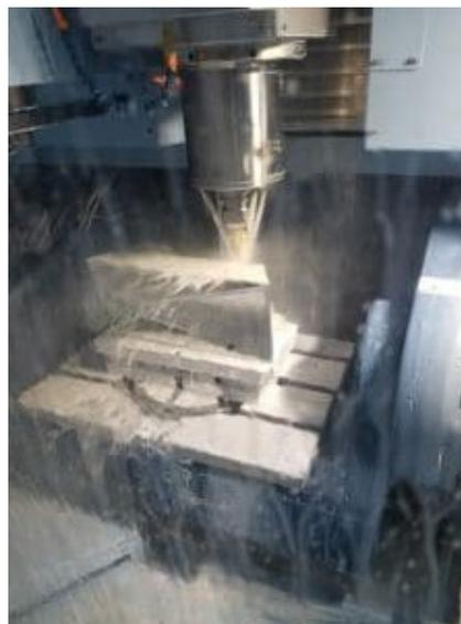
**High Torque retention knobs from JM Performance Products, along with dual-contact spindles and a combination of high-speed and conventional toolpath approach, have reduced cycle times as much as 40–50% for machining exotic materials like titanium, stainless steel and aluminum for Delta Machine’s aerospace, medical and automotive customers.**
