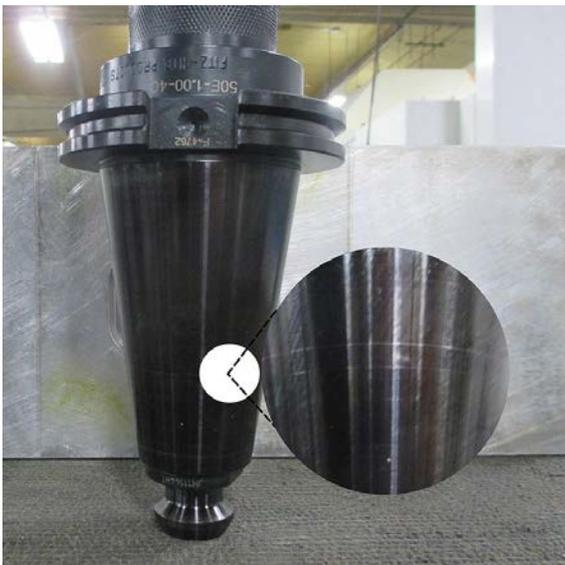
*Improper seating of the toolholder in the spindle due to poorly designed retention knobs often shows in uneven patterns visible on the taper.*
