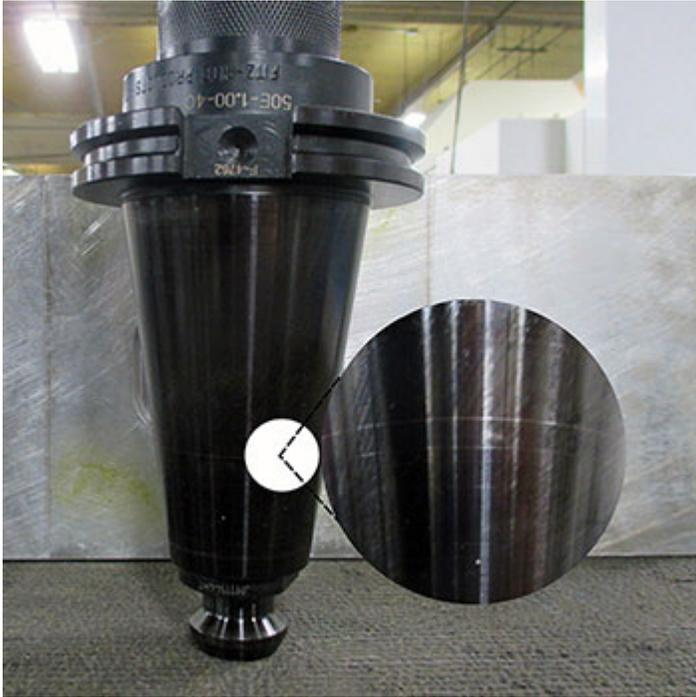
**Improper seating of tapered toolholders in the spindle can affect tolerances and precision, shorten tool and spindle life and even increase power consumption. Still, it is often overlooked as a factor in the performance and efficiency of CNC milling equipment.**
