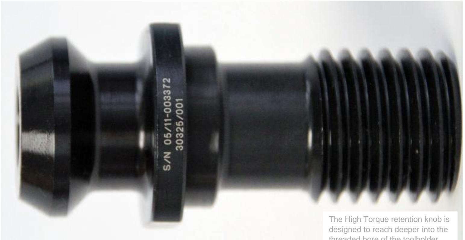
The High Torque retention knob is designed to reach deeper into the threaded bore of the toolholder. As a result, all thread engagement occurs in a region of the toolholder where there is a thicker cross-section of material to resist deformation.
