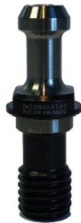
High Torque retention knobs are longer than a traditional retention knob but share the same head dimensions. The additional length also increases durability of the retention knob; a standard knob has less shank elasticity and will fatigue faster. Photos courtesy of JMPP
