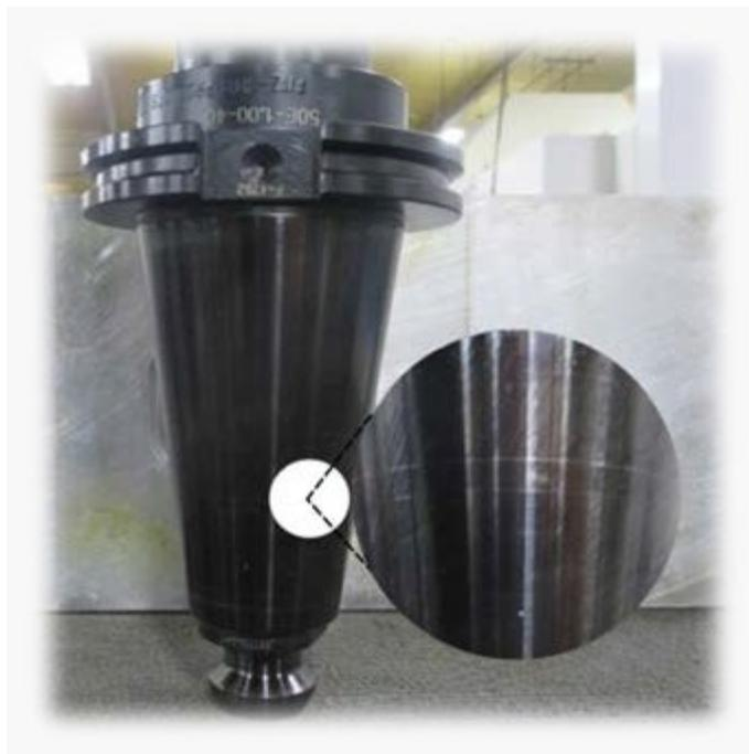
chatter, caused by a lack of concentricity, can be damaging to the spindle and the draw bar of the mill. With the advent of today’s very fast, very powerful, small footprint machines, this damage can directly result in the high-risk, red-flag safety dangers associated with a tool breaking loose during a cutting operation. In essence, it’s a disaster waiting to happen because if anything breaks loose—it would essentially be like a missile coming off the machine!
