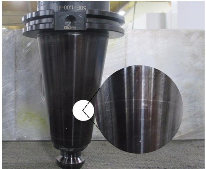
This case study from [JM Performance Products, Inc.](#) shares the success of an inexpensive fix for a flaw in the design and use of retention knobs in tapered toolholders secured by drawbars.
