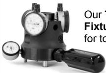
Our **Taper Shank Test Fixture** is used to check for toolholder distortion.
