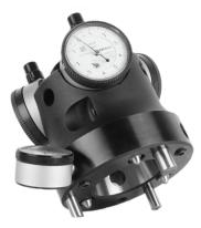
The Taper Shank Test Fixture is ground to mirror the taper of a CNC spindle. It measures the change of diameter by monitoring any movement of the toolholder perpendicular to the axis of the toolholder. The indicators measure movement of the toolholder in increments of 1/10,000 of an inch. The AT3 grind limit is .000059". Two graduation lines on the Taper Shank Test Fixture dial = .000058".
