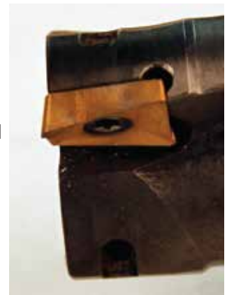
Observed Insert Wear After 93.4 Cu In Of Material Removal
