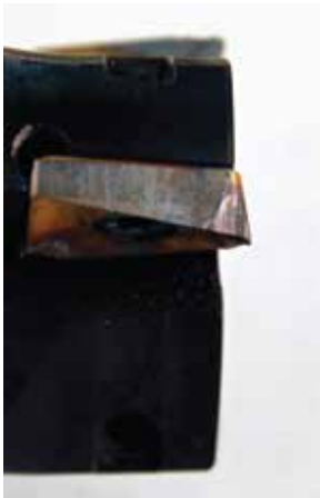
Observed Insert Wear After 93.4 Cu In Of Material Removal
