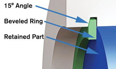
For applications in which end-play must be rigid, specify Rotor Clip VHO/VSH retaining rings.
