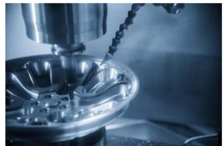
*The CNC milling machine or machining center cutting the mold part. Injection mold insert making by CNC machine.*
