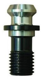
JMPP's High Torque knob is longer and reaches deeper into the cross section of the holder's threaded bore. As a result, all thread engagement occurs in a region of the toolholder where the cross-section is thicker to resist deformation, increasing rigidity and tool life.
