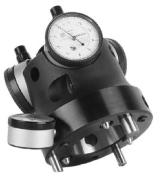
In an effort to ensure optimal mill productivity and tooling performance, JM Performance Products Inc. developed the Taper Shank Test Fixture, to check toolholders and test for taper deformation.
