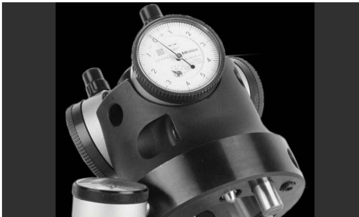
JM Performance Products Inc.'s Taper Shank test fixture performs tests on a toolholder with a retention knob already installed.
