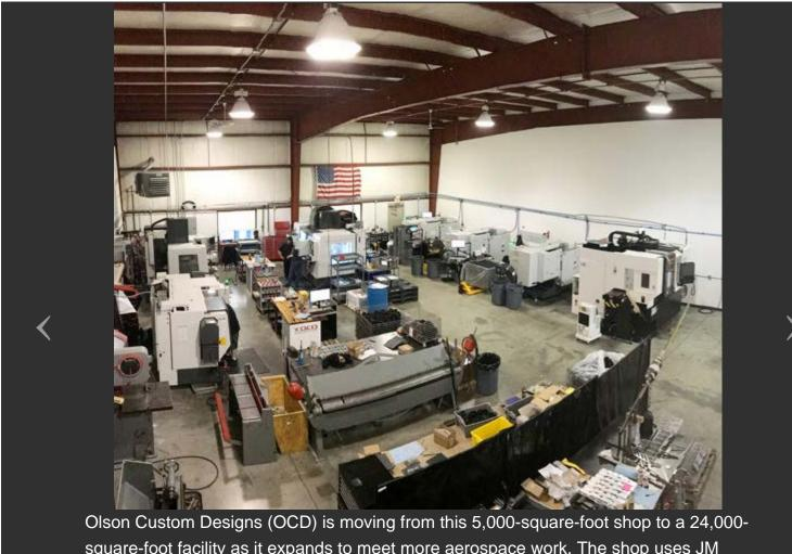
Olson Custom Designs (OCD) is moving from this 5,000-square-foot shop to a 24,000-square-foot facility as it expands to meet more aerospace work. The shop uses JM Performance Products' (JMPP) high-torque retention knobs on all of its 40-taper machining centers in order to achieve the accuracy required for aerospace quality standards.
