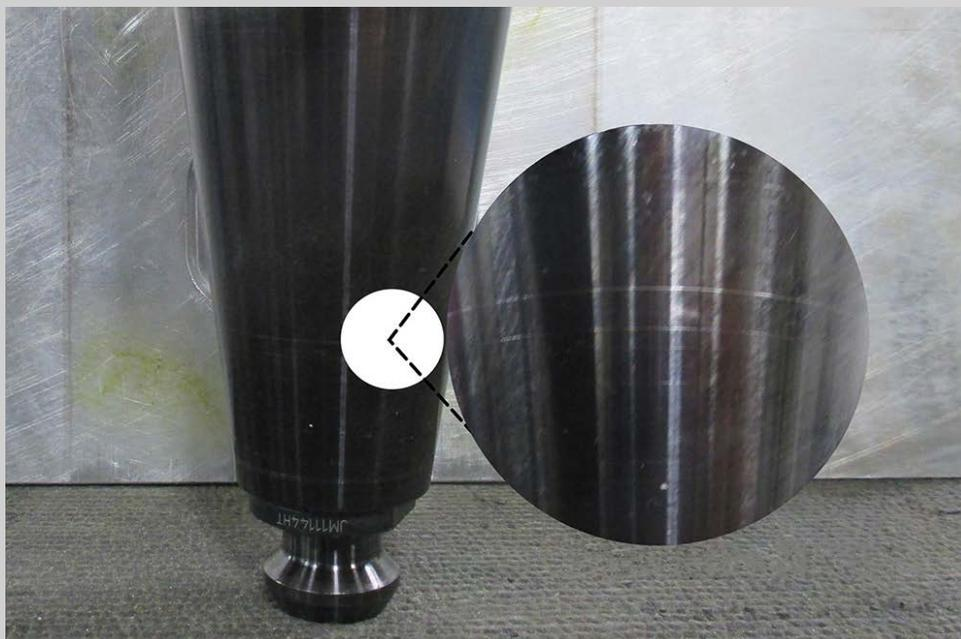
*JM Performance Products offers patented high-torque retention knobs designed to reduce or eliminate toolholder expansion responsible for costly and ongoing CNC milling and boring issues.*
