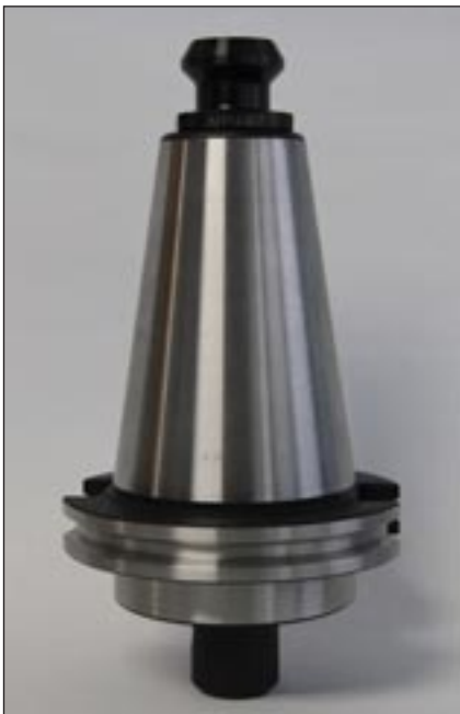
The High Torque retention knob installed in a toolholder. The knobs are longer to reach deeper into the threaded bore of the toolholder.
