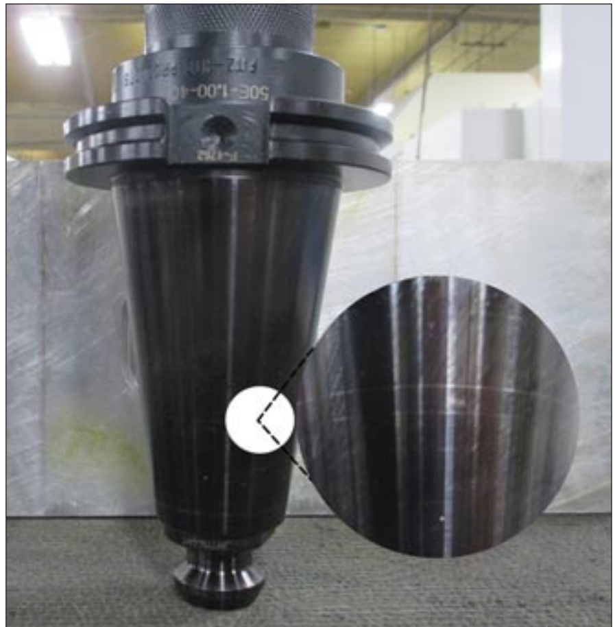
Toolholder wear is often attributed to other causes.
