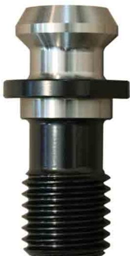
In fact, the problem of machine vibration and chatter is so common in CNC operations that use drawbars to hold tapered toolholders securely in the spindle that many are adopting a policy of selling only one style, the High Torque retention knob, or at least encouraging customers to invest a few dollars more for that item, one that many of do not offer.
