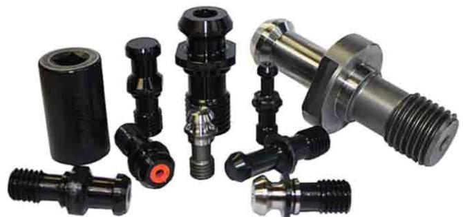
The High Torque retention knob is designed with a longer reach, so that it threads deeper into the threaded bore of the toolholder. Consequently, all thread engagement happens in an area of the toolholder where there is a denser cross-section of material to counter deformation.
