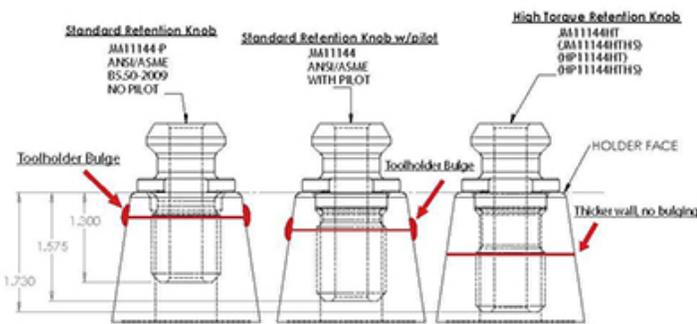
That is because when a standard retention knob is tightened, it can produce a bulge in the taper that prevents full contact and correct seating in the spindle. As a result, the toolholder is unable to pull completely into the spindle, and consequently cannot make contact
