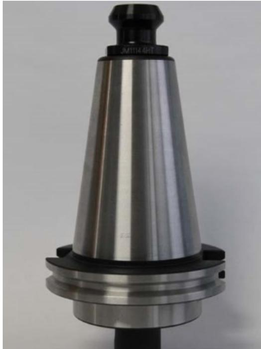
A High Torque retention knob installed in a toolholder. The retention knob is reported to work with existing toolholders, such as BT, DIN, ISO, and CAT toolholders, from 30 taper to 60 taper. Photo courtesy of JM Performance Products.
