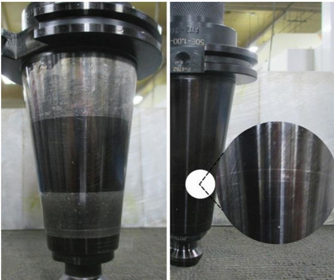
Hansen Engineering Co. used a standard retention knob in the toolholder on the left. Taper deformation prevents the toolholder from properly mating with the CNC machine's spindle, however. In contrast, the photo on the right shows use of JM Performance Products' high-torque retention knobs in the toolholder. A longer design enables the knob to reach deeper into the holder's threaded bore, improving taper-contact quality.
