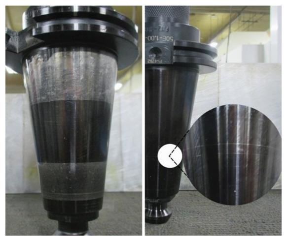
Hansen Engineering Co. used a standard retention knob in the toolholder on the left. Taper deformation prevents the toolholder from properly mating with the CNC machine's spindle, however. In contrast, the photo on the right shows use of JM Performance Products' high-torque retention knobs in the toolholder. A longer design enables the knob to reach deeper into the holder's threaded bore, improving taper-contact quality.
