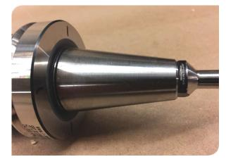
The solution was JMPP's patented High Torque retention knob, which works by making the retention knob as long as possible to fit the toolholder. It also includes a precision pilot, increases the undercut length and designs the threads to be balanced. When properly installed with a retention knob socket and torque wrench, this patented design prevents toolholder deformation.
